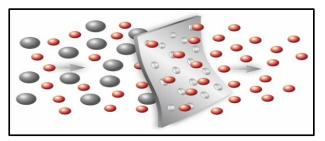
strip out chemical components that are considered undesirable contaminants or reduce the overall calorific value of the gas thus dropping the overall product value. In some instances, where  $CO_2$  and/or  $N_2$ removal is required, membrane technology may be employed.
