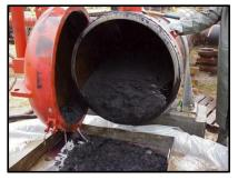
may contain significant concentrations of mercury. For some of these, the presence of mercury is expected, for example, the mercury bed media at end of life will contain high percentage concentrations of mercury and should be disposed of through approved routes; however, for some wastes, it may not be recognised that these could potentially be high in mercury (sometimes % levels) and should be treated as mercury waste. Some examples of these are:
